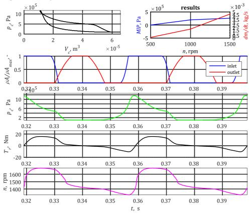
Fig. 5. Example of calculation results (2 cycles, 1500 rpm, *IVO* = 50 deg *BTDC*)
